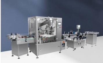
This machine has the functions such as automatical screw type bottle feeding, bottle detecting (no bottle no filling, no bottle no cap feeding), filling, cap feeding and capping automatically.
