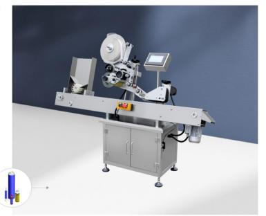
Top and bottom sides automatic labelling machine is suitable for label lesser height of square, round, and flat bottles in the industry of foodstuff, medicine, cosmetic and so on.
