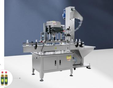
This automatic machine suit for sealing of disposable aliuminum wring type anti-theft caps. It can automatically arrange caps, drop caps, sleeve caps, capping head use hard stainless steel, use fourwheel balance principle, uniform force, with high quality. Star wheel equip with automatic clutch, if bottle locked it can stop working automatically.
